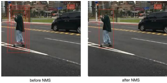
Figure 1 Schematic diagram of pedestrian detection and NMS combined repeat area
